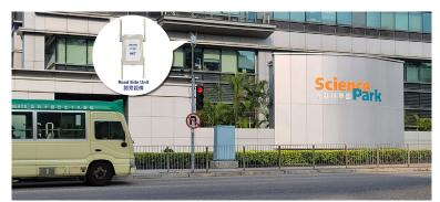
C-V2X road side units (RSU) are installed on traffic light poles and lamp posts along the designated route for providing real-time traffic intelligence to on-board units (OBU) installed inside the vehicles.
